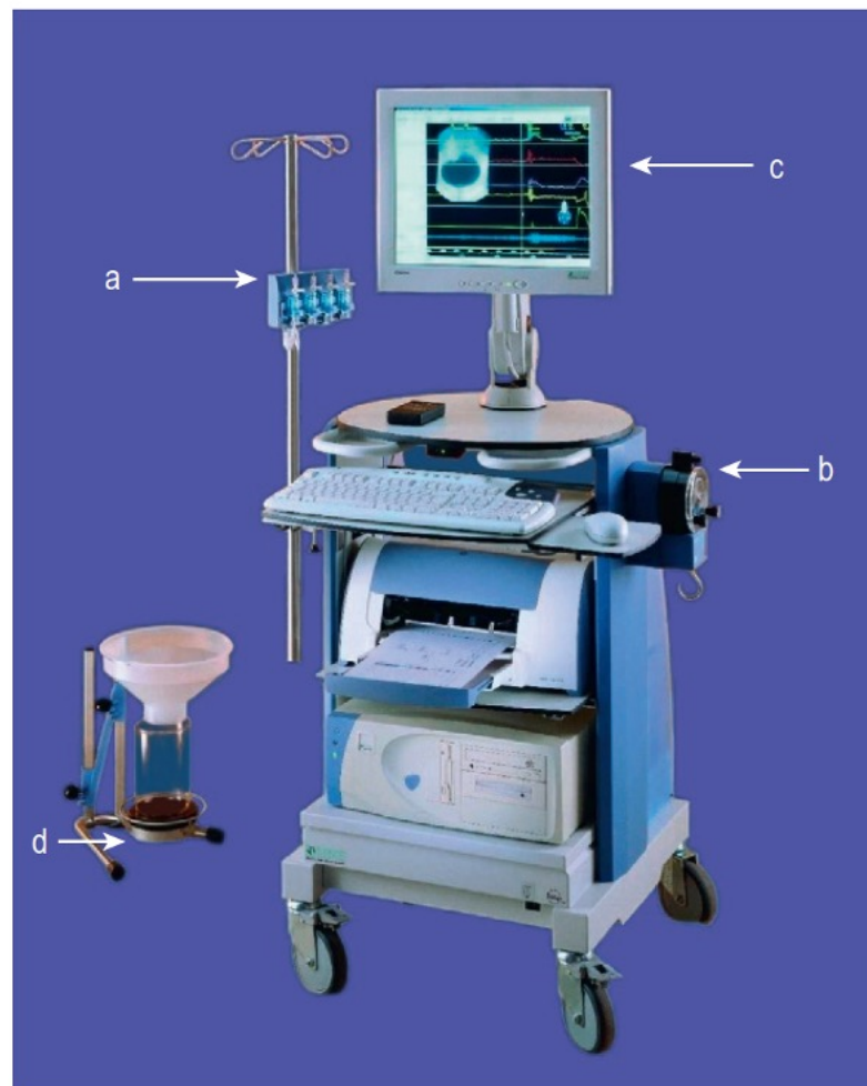
Fig. 4.2 Typical pressure flow workstation. The workstation comprises transducers on an adjustable-height stand ( a ); a pump for bladder filling ( b ); a display, in this case with a superimposed screening image ( c ); and a uroflowmeter for use during the voiding phase of the study ( d ).
