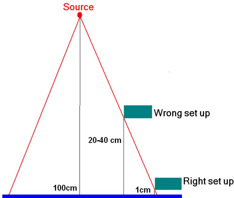
**Figure 1:** The lead shield used in electron mode, which is placed in various distances from the surface
