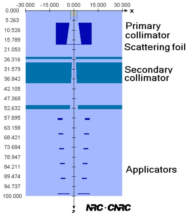
**Figure 2:** Simulation of the Linac's head using BEAMnrc. In electron mode, external applicators are attached to the head. The handmade shield should be placed after applicators, close to the surface.
